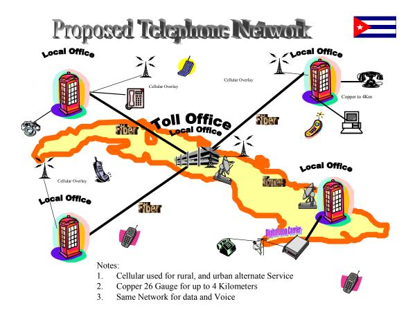
6. Item 5 discussed the cost of a wire-line network. A cellular network uses same switching components as the wire-line network but replaces the outside plant "feeder" and "distribution" network with radio transmission systems as discussed in detail in the "Cubacel" section of this report. The cost of providing individual wires to a fixed customer is much higher than cellular costs
